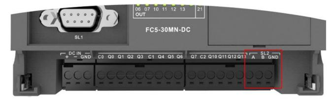
The pin definition of serial port 2 is as follows:
