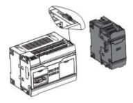
Step2. Then push the extension module into place against the mainframe interface and reverse the latch to lock the extension module.
