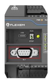
Serial communication port 1 is DB9 type and supports RS485 or RS232 communication with the pin definitions as follows.
