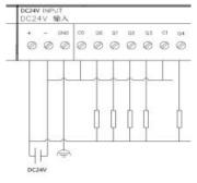
• PNP type (Source) transistor output wiring:
