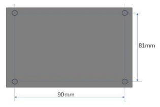
• The following diagram shows the mounting holes for the 40 points I/O CPU.
